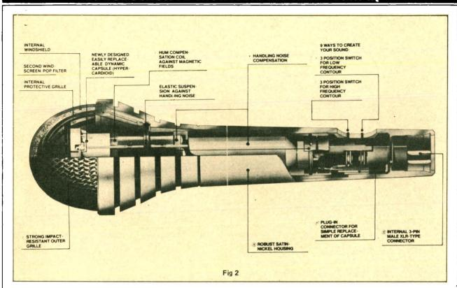
bass roll-off switch for this purpose. Additionally, aiming the microphone up, towards the singer's nose, will eliminate the nasal or "closed nose" effect.
